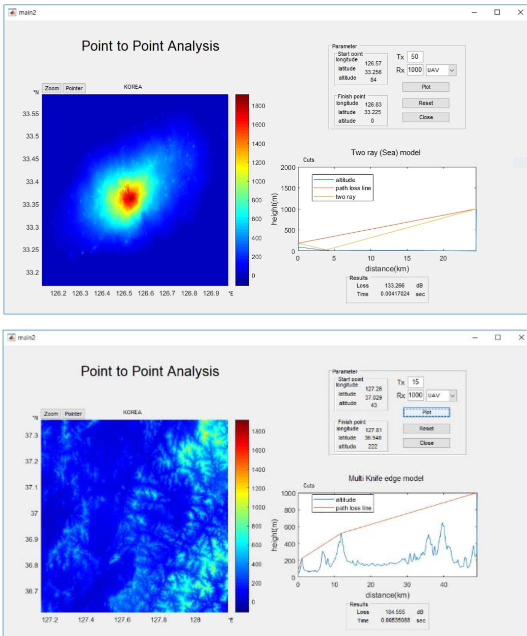
Fig. 8. Simulator 1: Checking the channel model between the transmitter and receiver (upper: under water, lower: mountainous)
