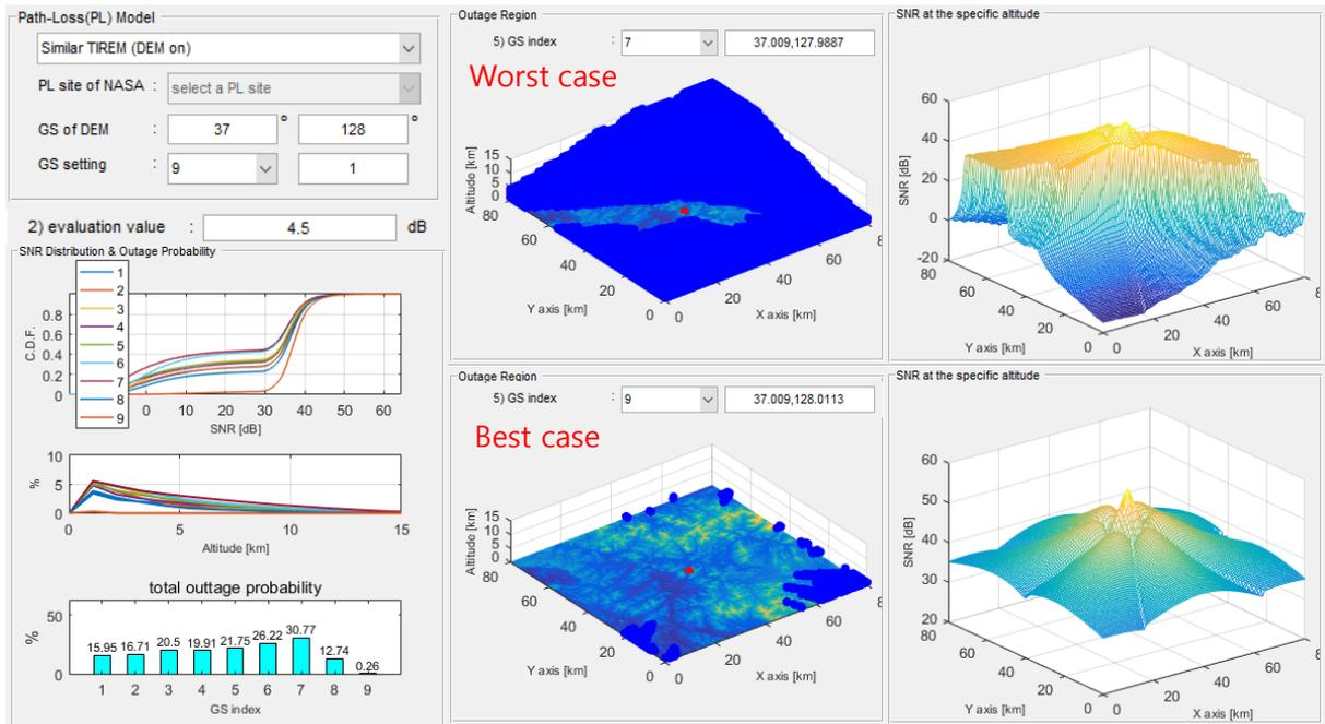
Fig. 10. Simulator 2: SNR analysis simulator for comparing various GS locations
