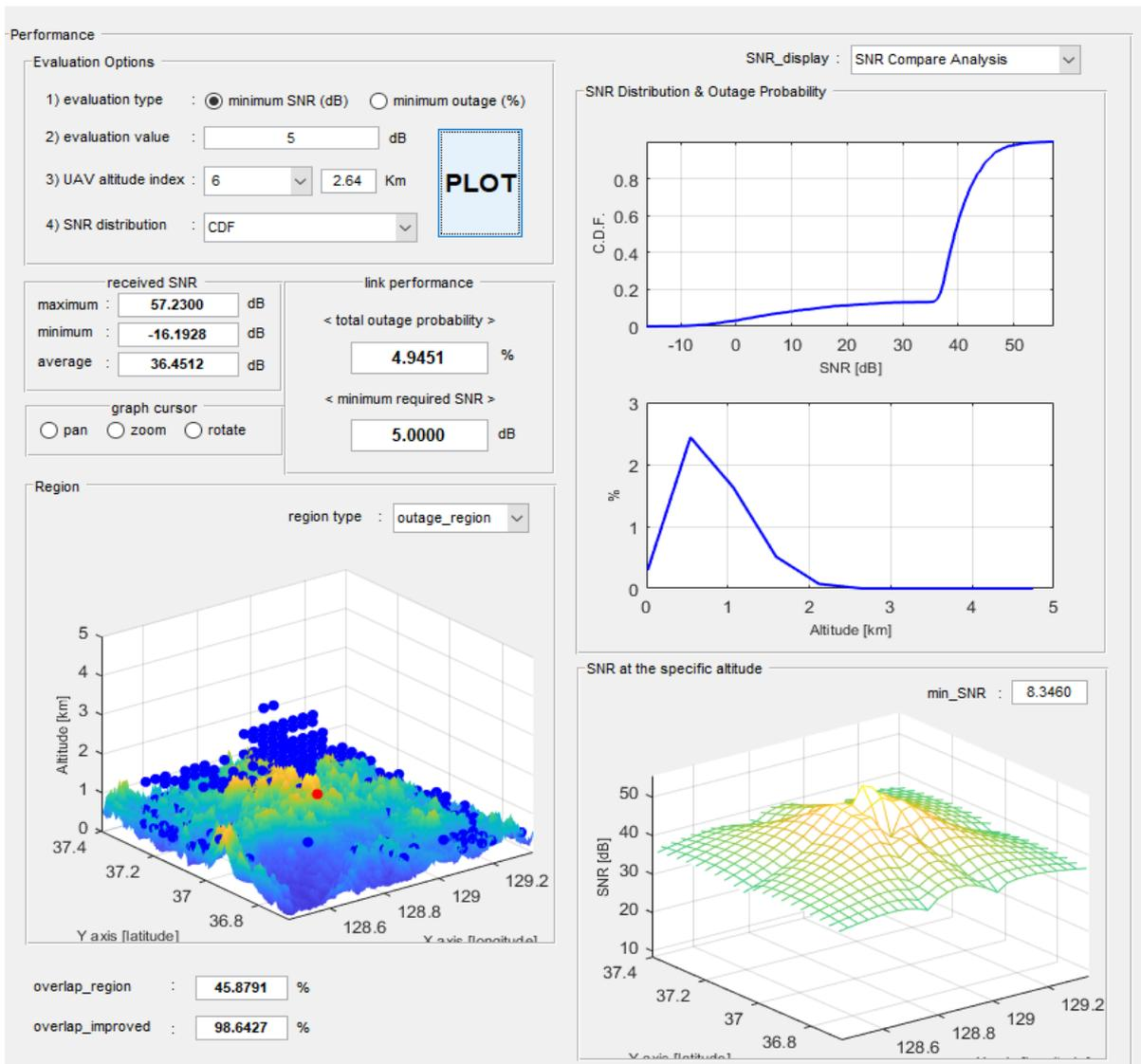
Fig. 9. Simulator 2: SNR analysis simulator for selecting a GS location
