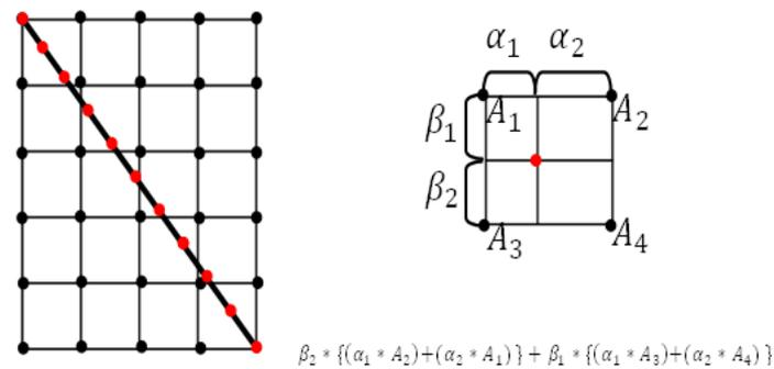
Fig. 4. Interpolation method of DEM
