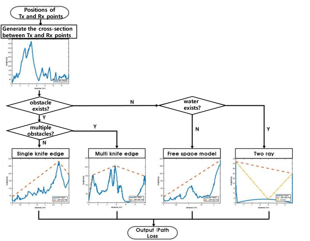
Fig. 6. Channel model selection algorithm
